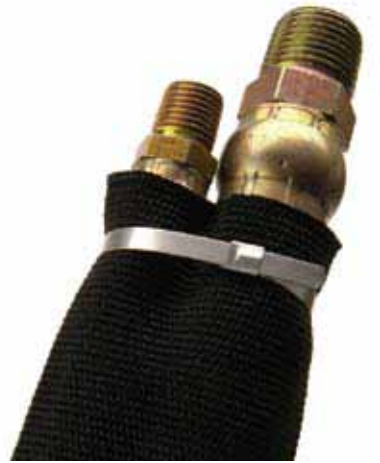
Multiple high pressure hoses can be bundled tightly together to protect them from abrasion and weather, and to protect personnel from potential harm due to high pressure rupture.
